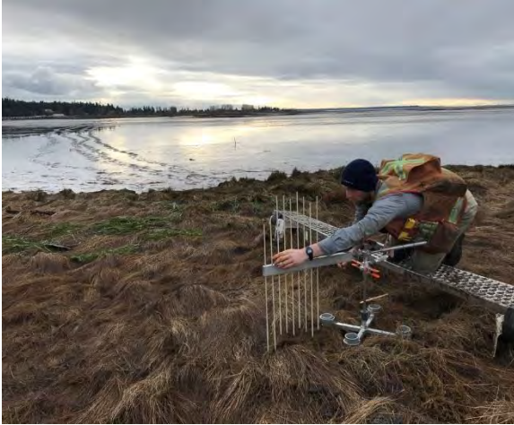
Figure 2 Photo of installed rSET and measurements being taken
