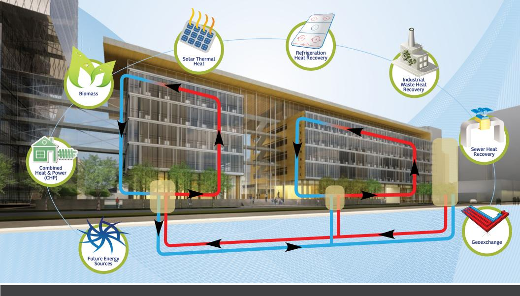
The district energy system to service new City Hall captures energy by utilizing a vertical, closed loop geoexchange system that uses heat pumps to store and extract heat from the ground underneath the parkade that has been constructed as part of the new City Hall / Community Plaza Project.
