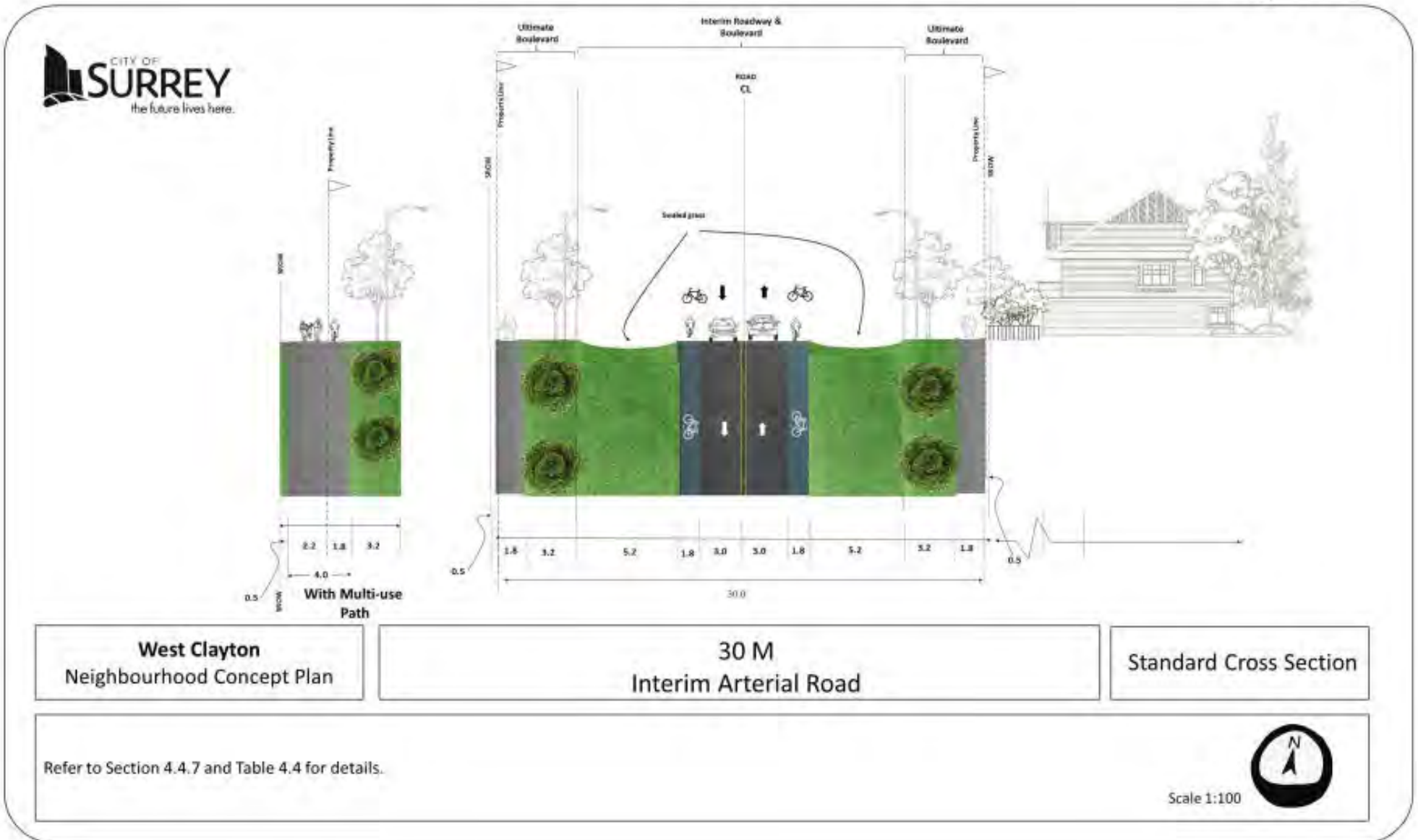
Figure 4.13 - Interim Arterial Road Standard
