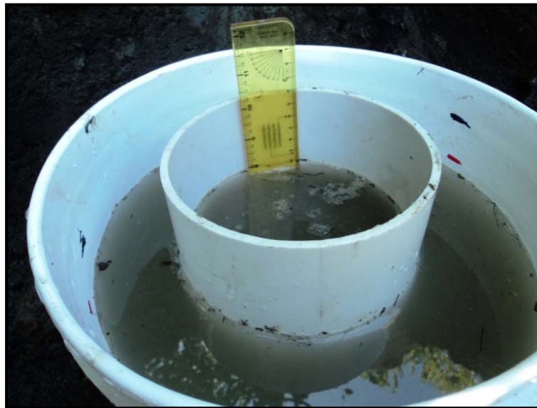
Fig 2. Double-ring infiltrometer setup.
