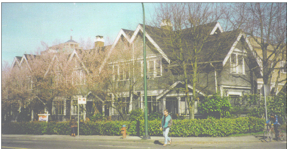
The character of medium density stacked townhouses, row housing and apartment buildings can convey a single family residential atmosphere to the street. The use of gable roof components and clear identification of the front entrance to ground oriented units is a dominant characteristic.
