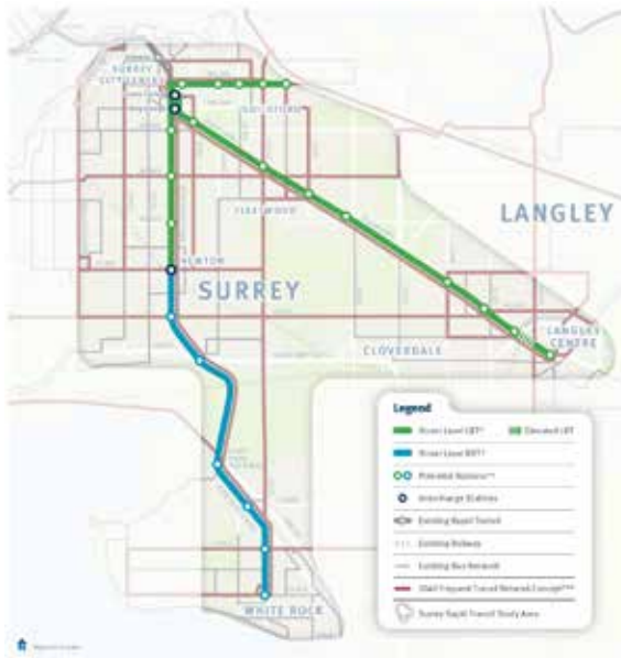
Figure 22: Preferred Rapid Transit Future: Surrey's preferred option within TransLink's option analysis is light rail from City Centre to three town centres: Guildford, Langley City and Newton; and Bus Rapid Transit from Newton to White Rock City Centre. (Map: TransLink / Ministry of Transportation and Infrastructure)
