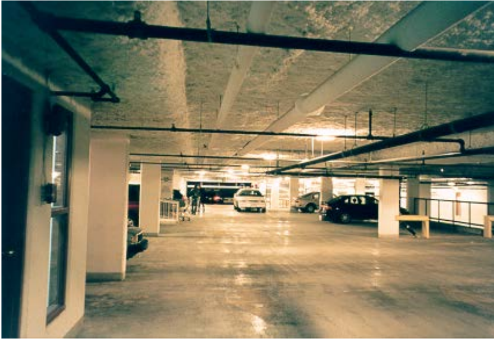
Walls and columns painted white, bright lighting, glazed elevator core, and transparent railings.
