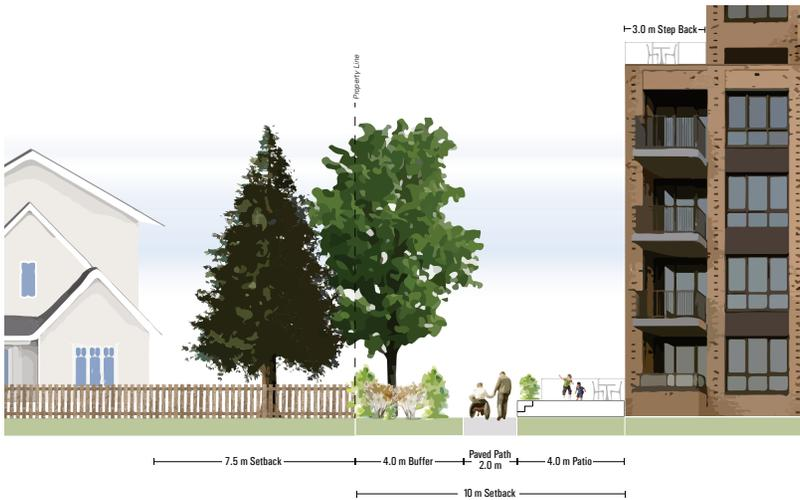
FIGURE 4.4.4B LOW-RISE APARTMENT TO LOW-DENSITY RESIDENTIAL (SIDE OF UNIT)
