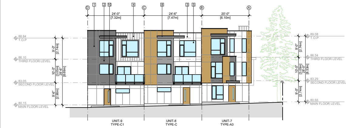
3 BUILDING-2 WEST ELEVATION Scale: 1/16" = 1'-0"
