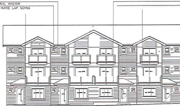
BLDG #3: NORTHEAST ELEVATION
