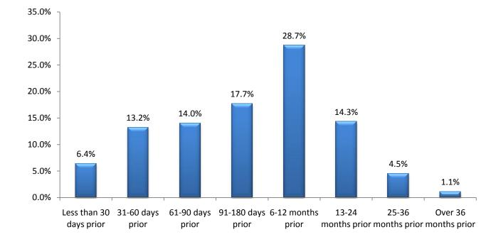
Figure 10: Length of Time between Last Inspection and Residential Fire (1988-2003; n = 265)
