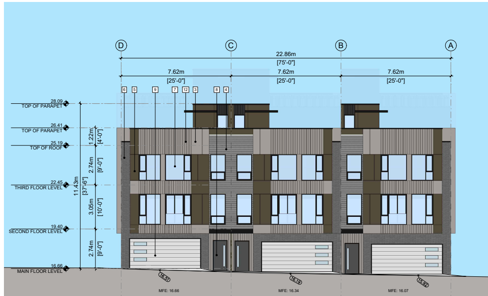
1 BUILDING 4 NORTH ELEVATION
