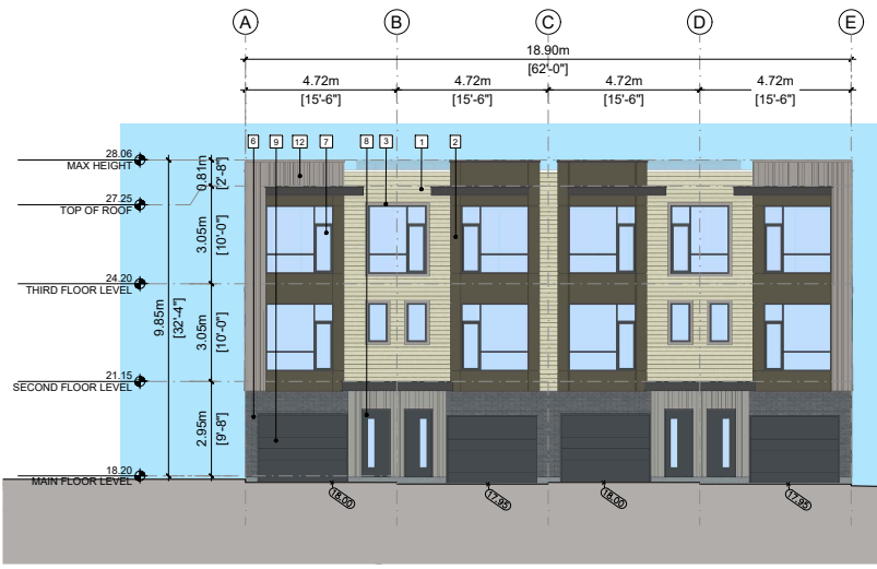
① BUILDING 11 NORTH ELEVATION
