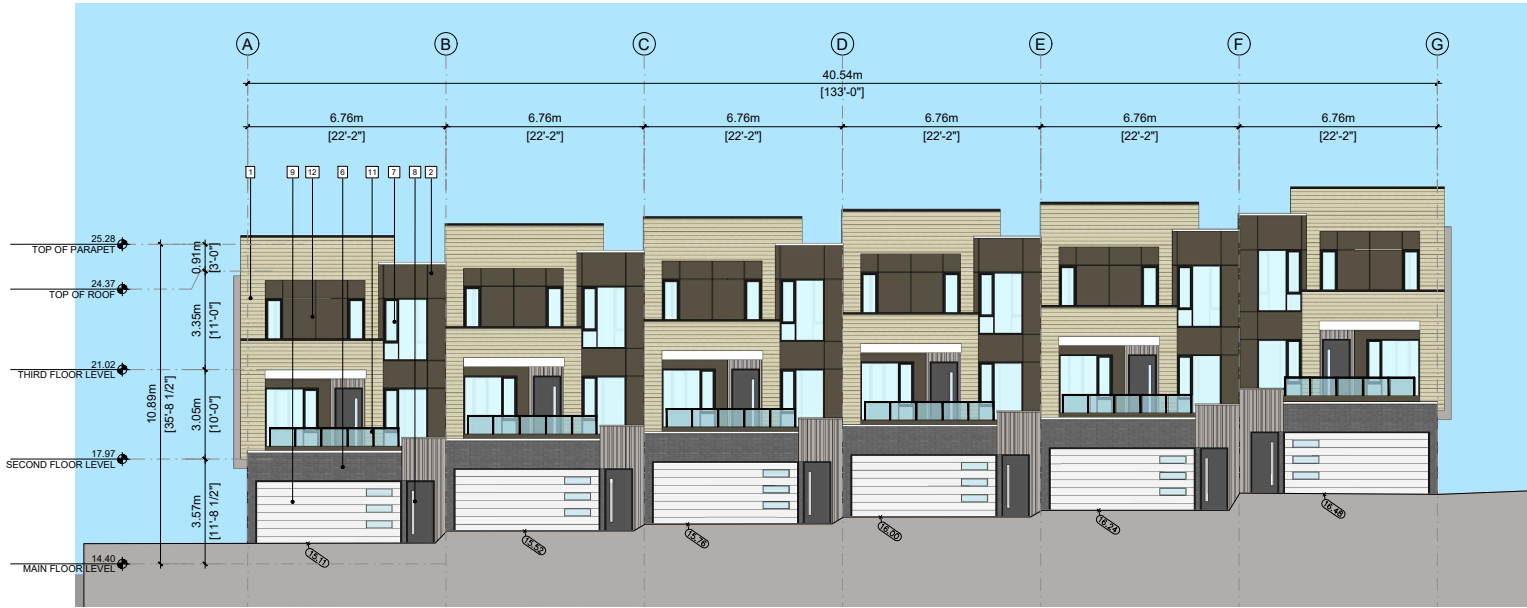
1 BUILDING 1 SOUTH ELEVATION
