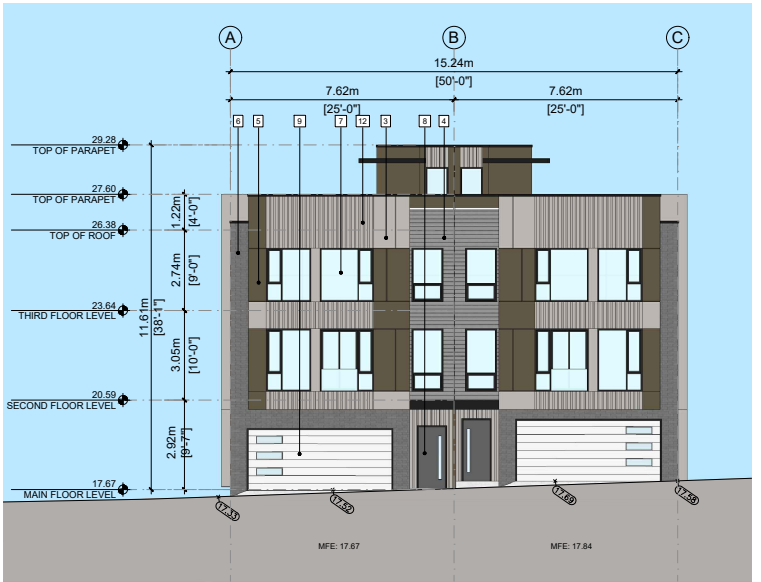
3 BUILDING 6 SOUTH ELEVATION
