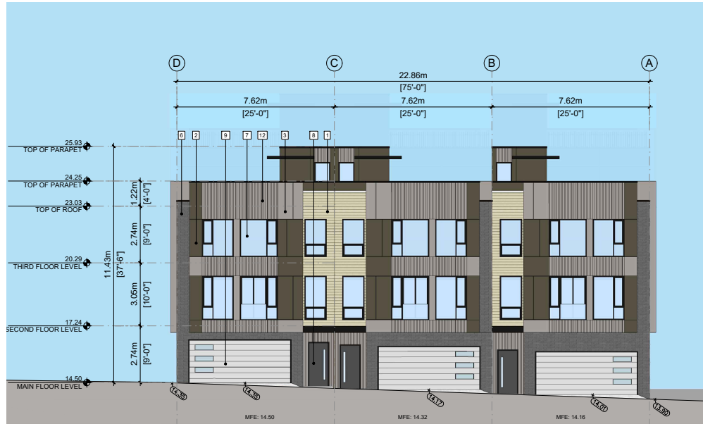
1 BUILDING 7 NORTH ELEVATION
