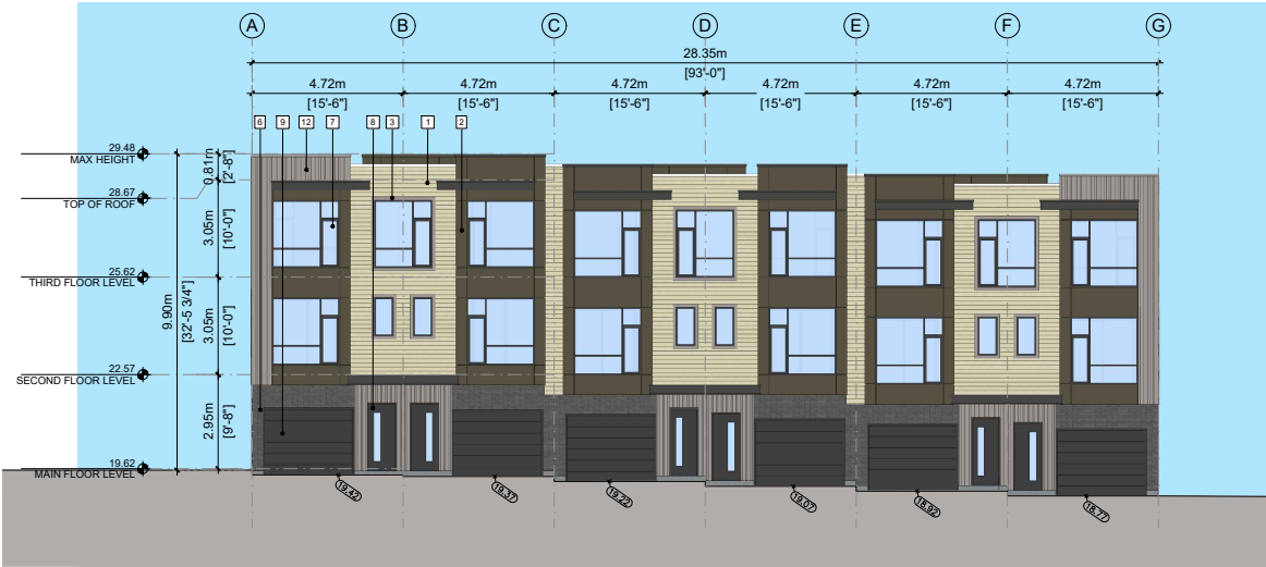
① BUILDING 9 NORTH ELEVATION
