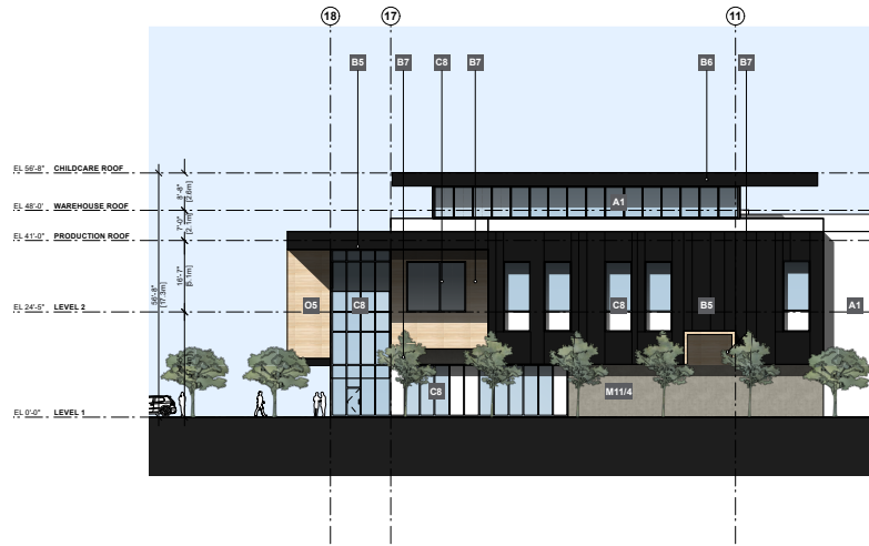
1 PARTIAL SOUTH ELEVATION 1/32" = 1'-0"
