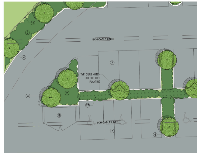
4 TYPICAL PLANTING ISLAND/ BIO-SWALE 1 : 100
