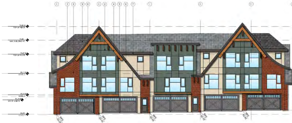
1 BUILDING 6 - WEST ELEVATION SCALE: 1/8" = 1'-0"
