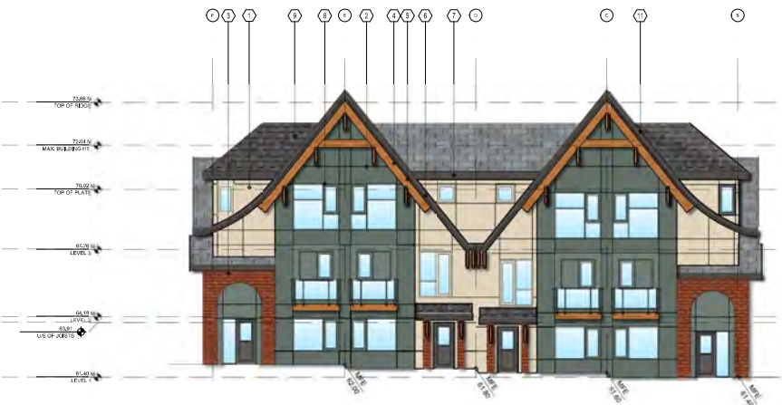
3 BUILDINGS 10 NORTH ELEVATION SCALE: 1/8" = 1'-0"
