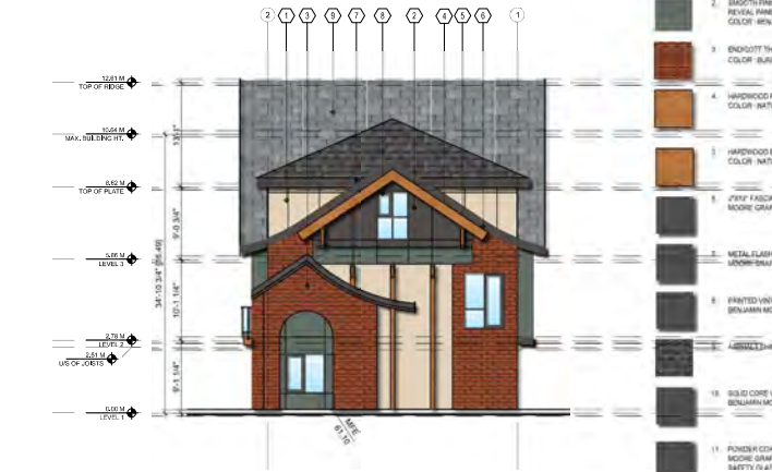
2 BUILDING 8- WEST ELEVATION SCALE: 1/8" = 1'-0"
