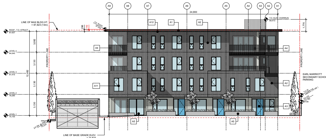
1 BLDG A - NORTH ELEVATION - MEWS Scale: 1:100
