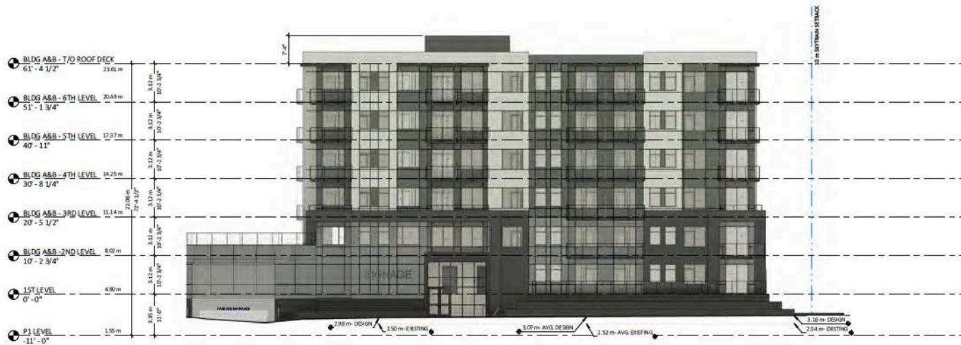
BUILDING B - WEST ELEVATION 3/32" = 1'-0"
