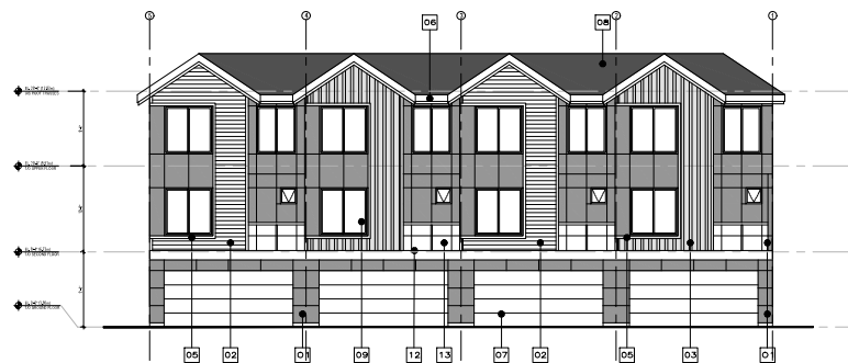
2 BUILDING 3 - NORTH ELEVATION 1/8" = 1'-0"
