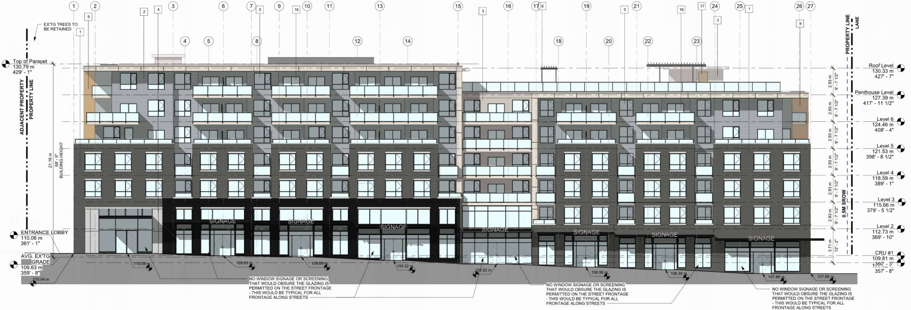
1 EAST ELEVATION (152 STREET) A-301 3/32" = 1'-0"
