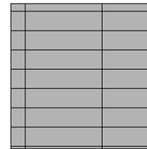
EXTERIOR HIGH DENSITY FIBRE CEMENT BOARD C/W EASY TRIMS TO MATCH (HARDIE OR SIMILAR) COLOR - LIGHT GRAY
