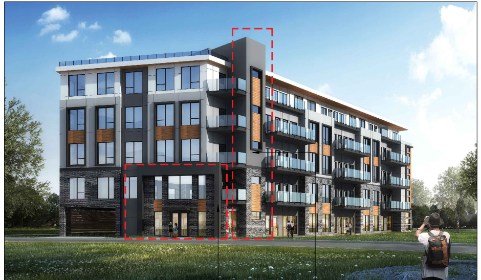
Brick + dark grey - Suggest strategies to accentuate the entryway as the current entrance lacks identification and appeal. - Dark grey frame - Recessed wall in brick - Narrow openings
