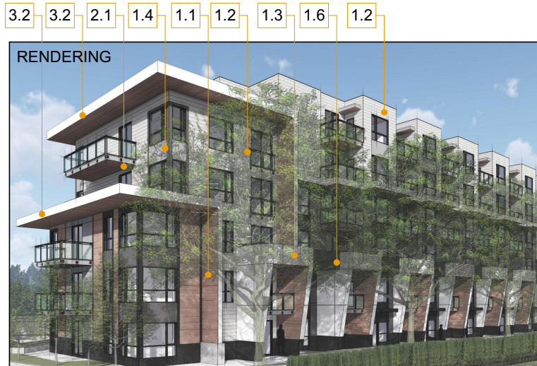
1.3 | Fibre Cement Panel w/ Reveal - Arctic White
