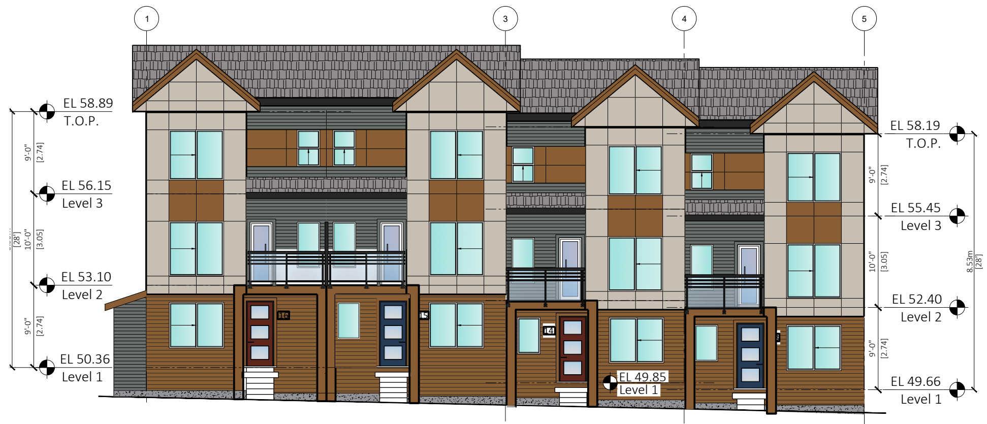
2 REAR (NORTH) ELEVATION 3/32"=1'-0"
