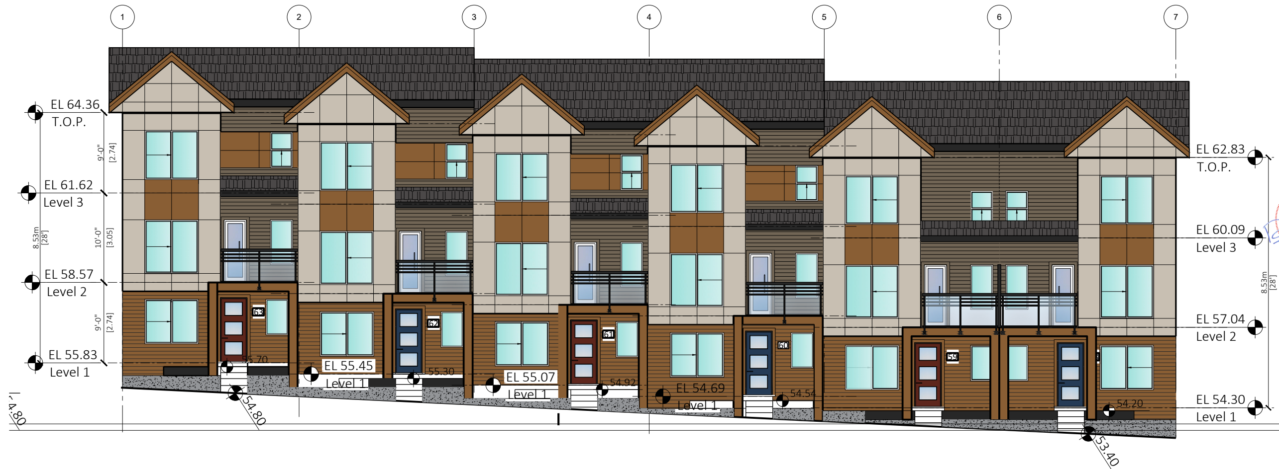
2 REAR (NORTH) ELEVATION 3/32"=1'-0"
