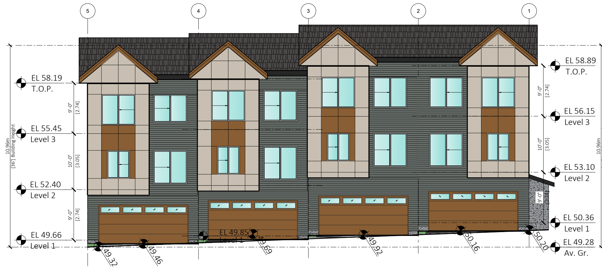
1 FRONT (SOUTH) ELEVATION 3/32"=1'-0"
