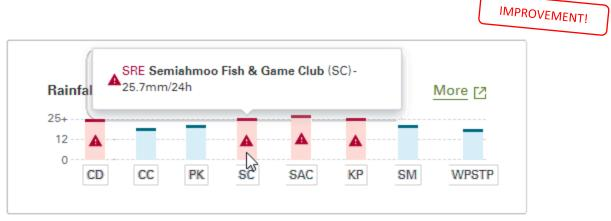
View of the rainfall widget showing how an SRE is displayed and the ability to query the current rainfall values for each station.
