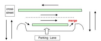
The second concept in Exhibit 4.1 is also a multi-way boulevard where one of the SB traffic lanes is converted into a parking access roadway behind a landscaped buffer boulevard, and on the NB the parking access roadway is simply added to three existing through traffic lanes. In addition to the issues discussed above, the following issues are also relevant:
