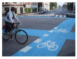
• On-street parking and curb bulges. The recommendations for the street network and parking both emphasize use of on-street space, especially during off-peak periods. These illustrations show how a curb lane has been set aside for parking with the curb extended at the intersection and near a crosswalk, to narrow the crossing distance for pedestrians. These are already being applied on some local and collector roads in the City Centre.
