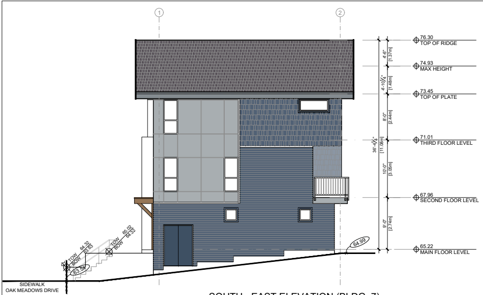
SOUTH - EAST ELEVATION (BLDG. 7)
