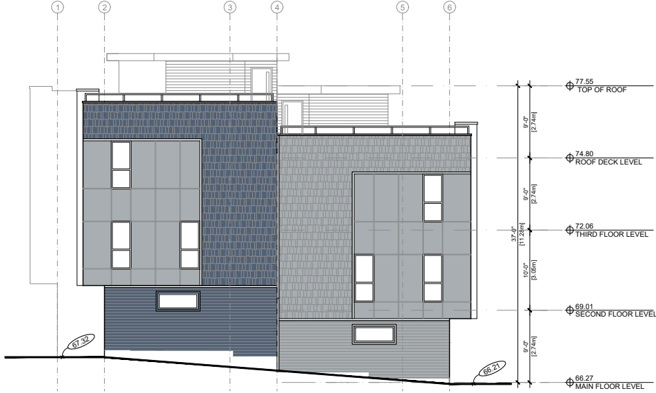
WEST ELEVATION (BLDG. 4)
