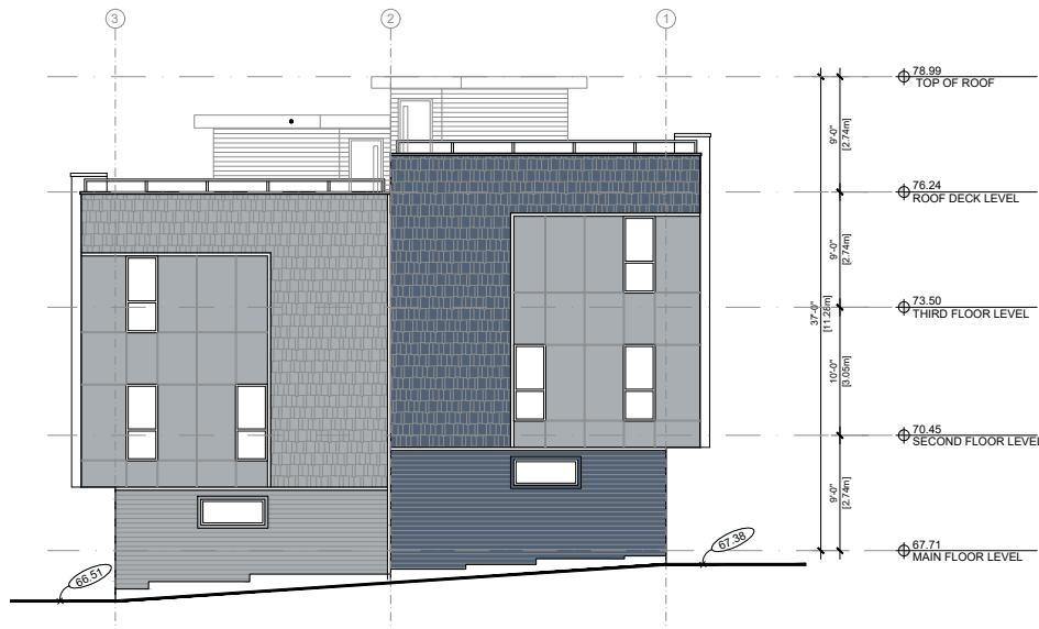
WEST ELEVATION (BLDG. 5) (ALONG 164 STREET)
