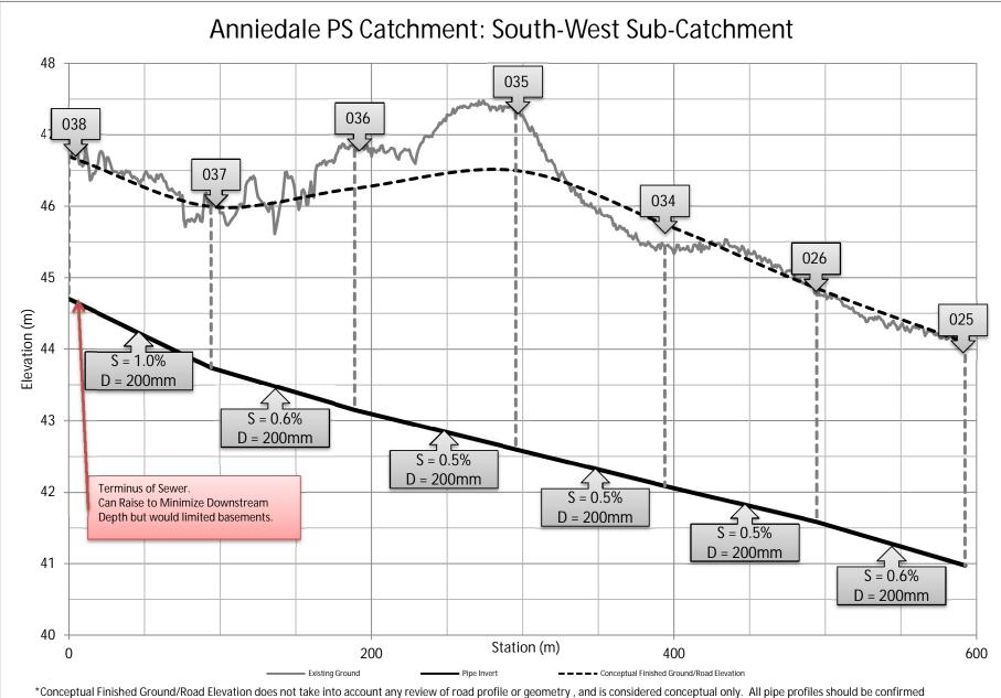
\*Conceptual Finished Ground/Road Elevation does not take into account any review of road profile or geometry, and is considered conceptual only. All pipe profiles should be confirmed once road profiles have been developed.
