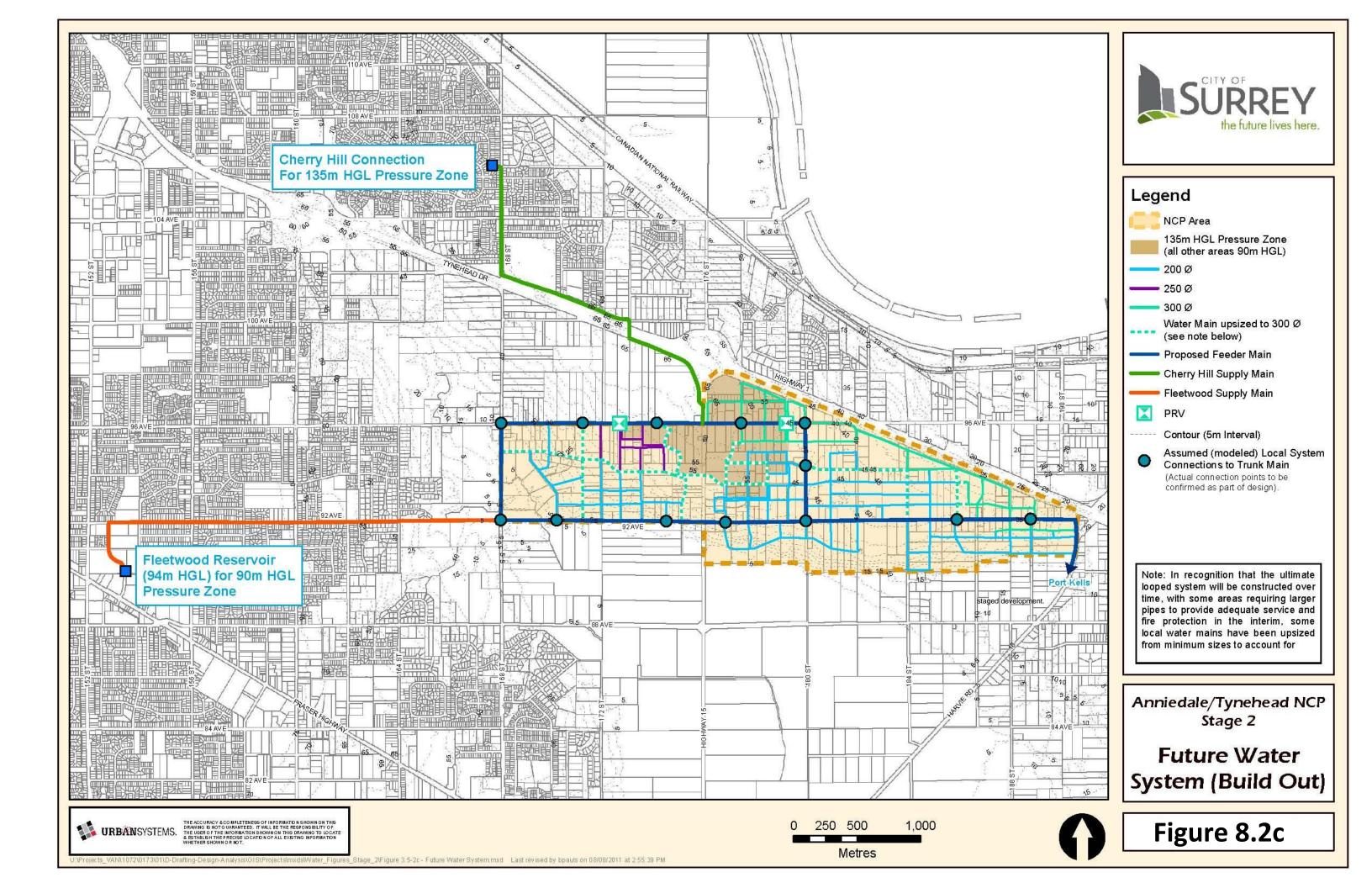
As the Fleetwood Reservoir has an estimated in-service date of 2017, any development occurring in the lower pressure zone prior to the new reservoir coming online could be fed through a PRV via the Cherry Hill Connection. This connection would be considered as a temporary supply source only. PRVs between the two pressure zones will remain in place for future conditions for emergency supply only, with no inter-pressure zone flow under normal demand scenarios.
