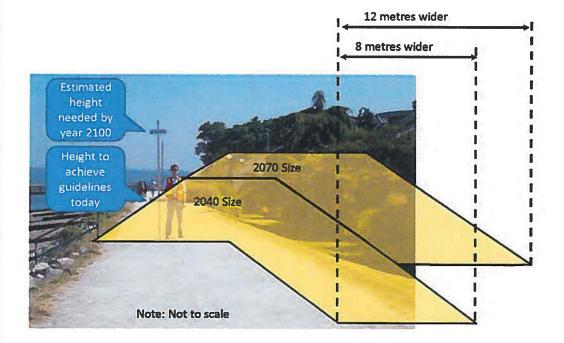
A possible dyke upgrade in Crescent Beach would need to be significantly higher and wider than the current dyke, especially by 2070.
