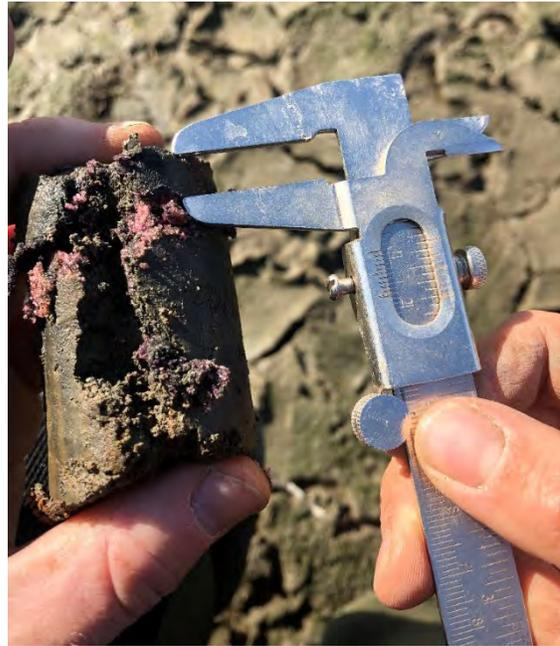
Figure 6. Marker horizon measurement being taken using vernier calipers. Marker horizon is the pink band below what is currently being measured between the caliper's external jaws.
