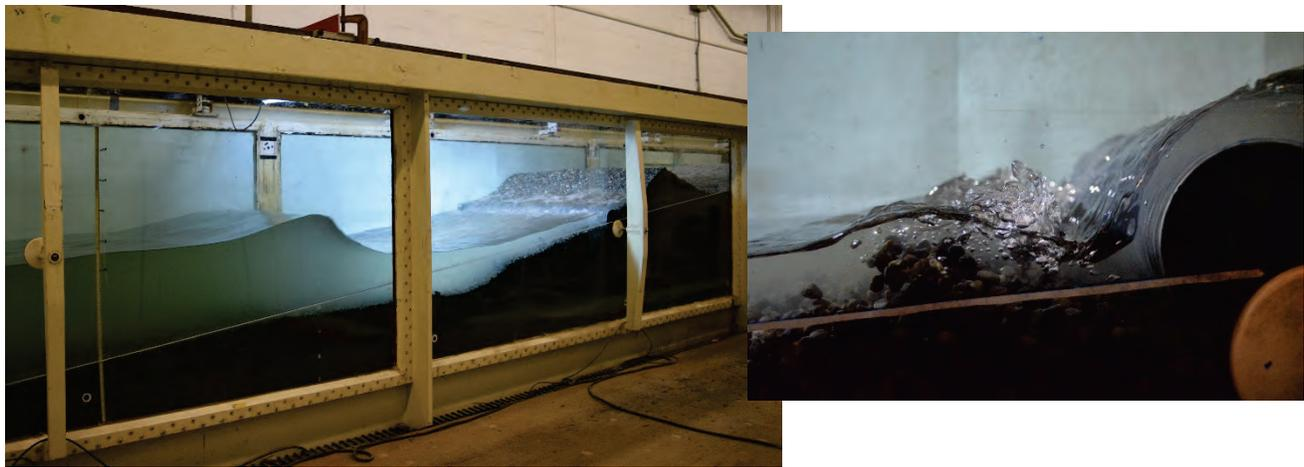
Figure 3.3 Photos of physical model studies undertaken by J. Wilson of the effects of woody debris on shoreline response during storm events at the National Research Council, Fall 2019 (J. Wilson, NHC)
