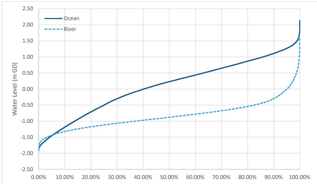
**Figure 1. Percentile plot of modelled ocean and river water levels at the current Serpentine sea dam for October (1964 to 2010).**
