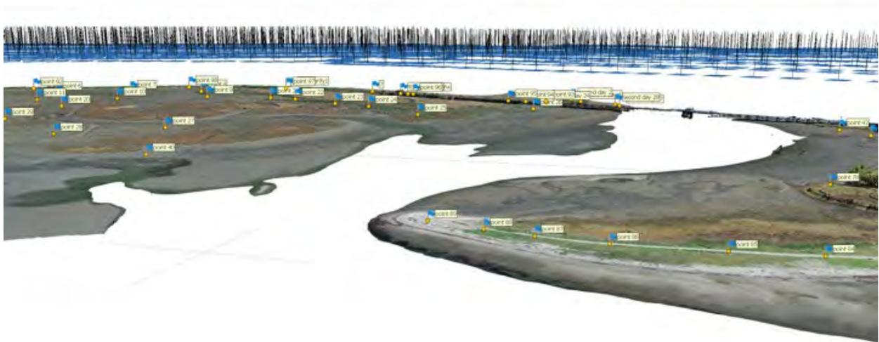
Figure 17 Photogrammetry is used to create a detailed 3D model of Mud Bay
