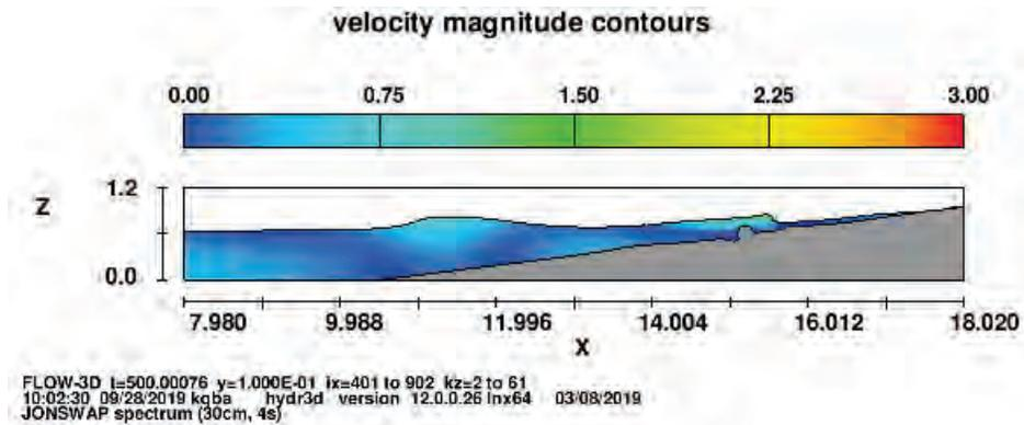
Figure 3.2 Output from a Flow3D CFD model of wave-shoreline interactions. (J. Wilson, NHC)
