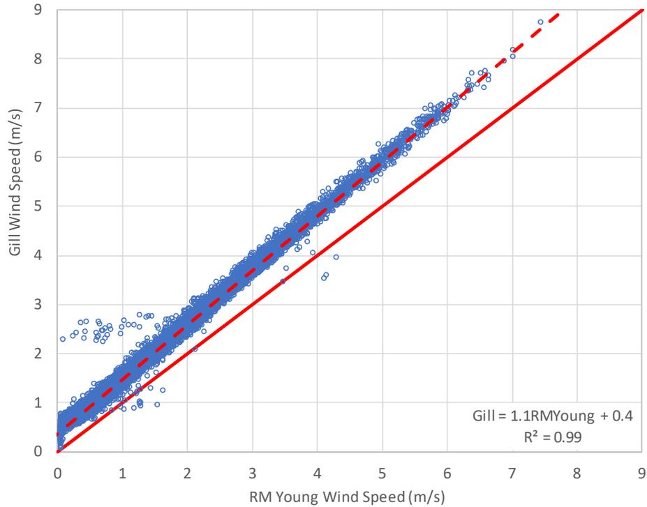
**Figure 3-2 Comparison of wind speed data during the 1 September to 31 October 2019 preliminary assessment period from the RM Young mechanical and Gill WindSonic ultrasonic wind sensors installed at the Colebrook Road Pump House Onshore Wind Monitoring Station. Data are 2-minute average values based on 3 second samples.**
