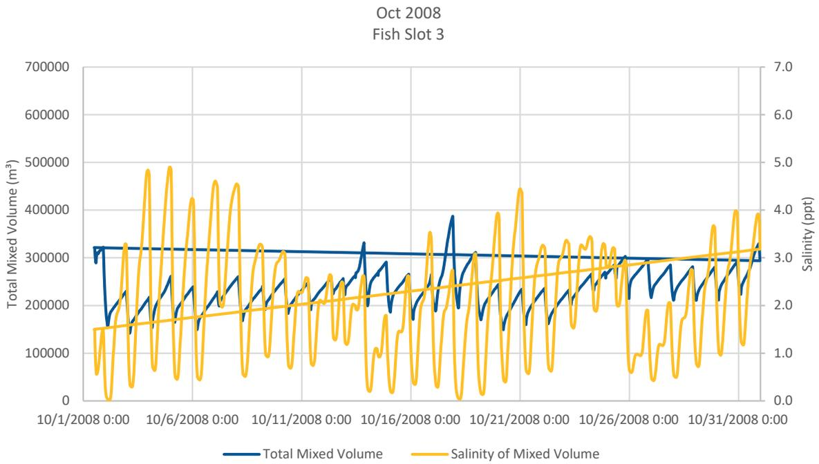
**Figure 3. Computed salinity of mixed volume of water 2.6 km upstream of relocated sea dam with fish slot 1 (above) and fish slot 3 (below).**
