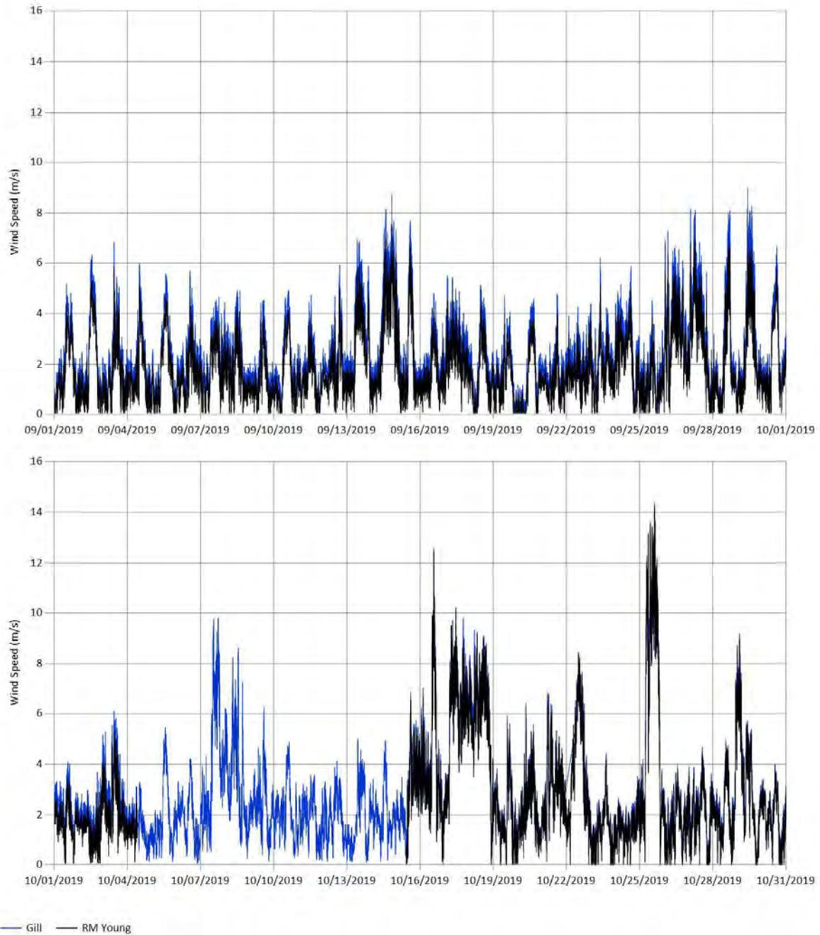
**Figure 3-1** Wind speed data during the 1 September to 31 October 2019 preliminary assessment period from the RM Young mechanical and Gill WindSonic ultrasonic wind sensors installed at the Colebrook Road Pump House Onshore Wind Monitoring Station. Data are 2-minute average values based on 3 second samples.
