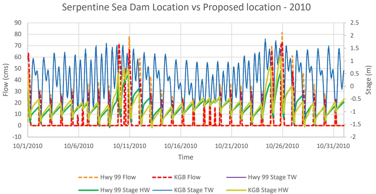
**Figure 2: Modelled water levels for different flood conditions for the current location (KGB) and the proposed location (Hwy 99) for the Serpentine Sea Dam**
