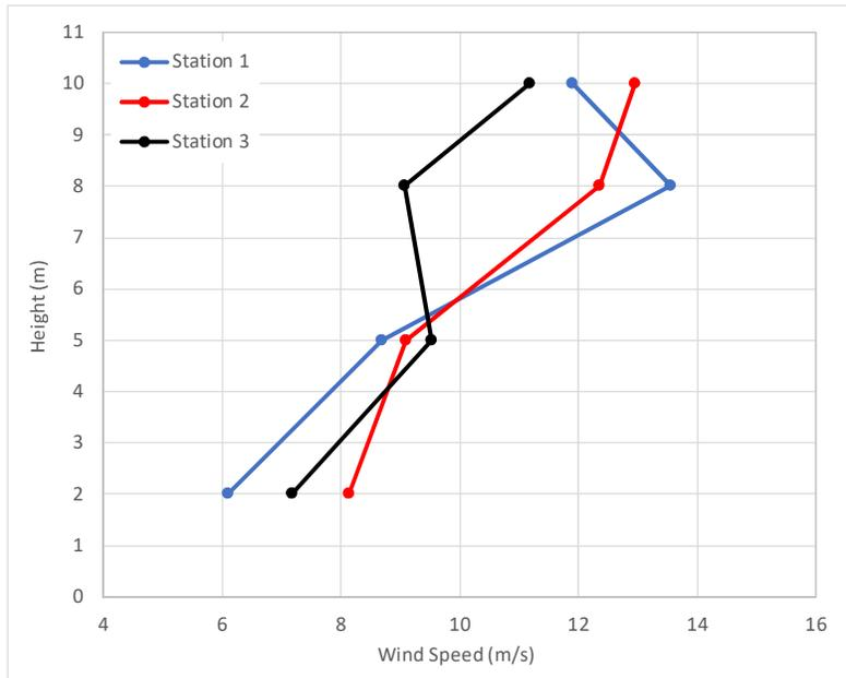
**Figure 3-5** Wind speed profiles during a moderate wind event on 25 October 2019, collected adjacent to the Colebrook Road Pump Station (station 1) and 110 m and 270 m west along the dyke road from the pump station (station 2 and 3 respectively).
