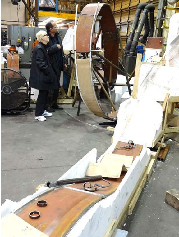
Fabrication of artwork using a 3D foam pattern to assist welder to form the complex curves.
