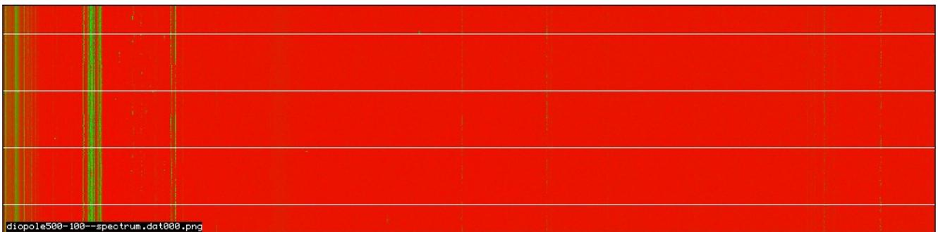
In this series of spectrum scans and a composite spectrogram, we see some signals in the HF region under 50MHz in the first division and some FM broadcast stations around 100MHz at the first division. There are no obvious signals generated by the HPS or MH lamps.
