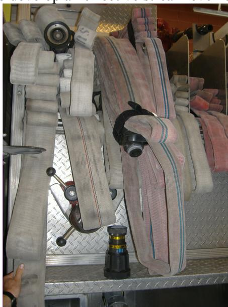
Figure 14 -- Surrey’s pilot standpipe pack relies on 1.75 inch hoseline with combination nozzle. Removal of nozzle tip creates a smooth bore pattern.
