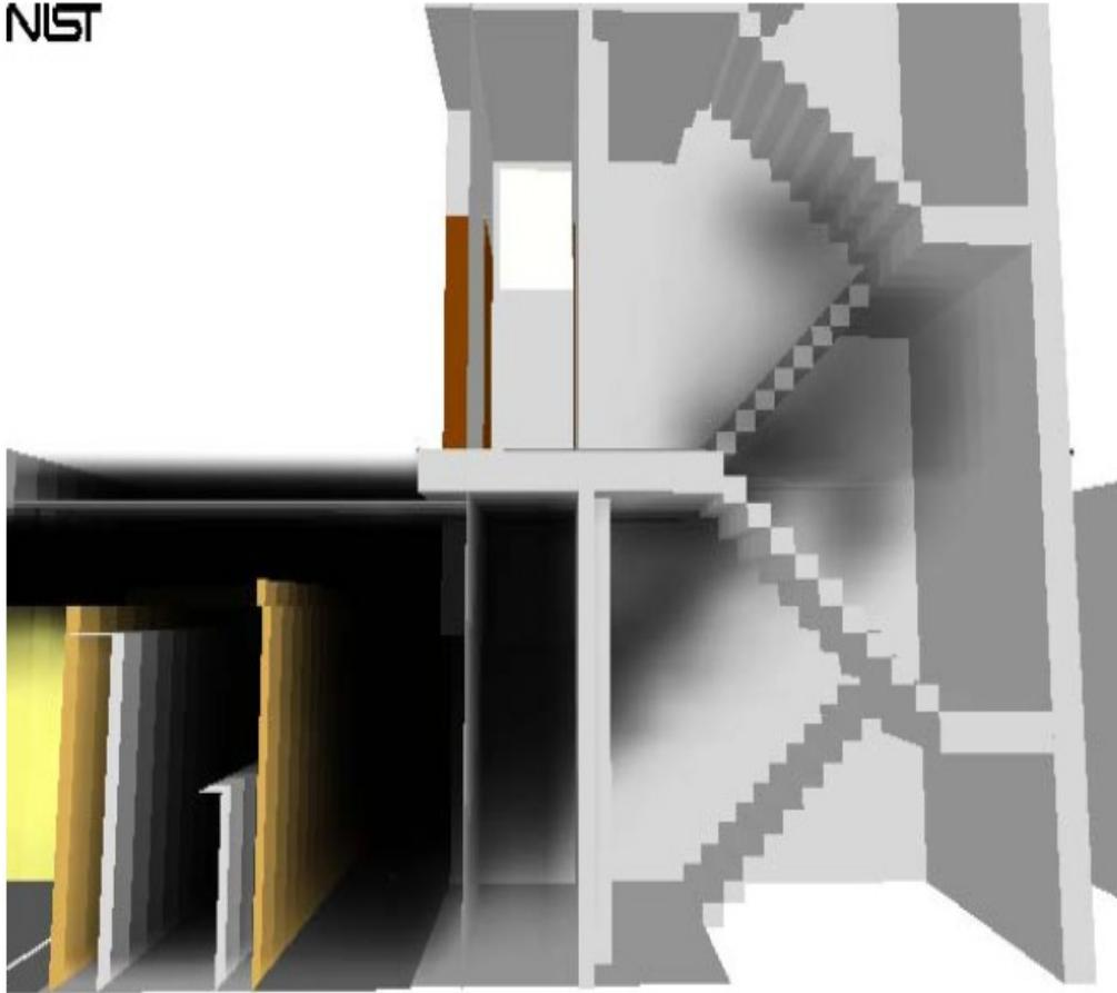
Figure 6a -- Cook County office building schematic showing infiltration of smoke from fire floor to stairwell. (NIST Graphic).
