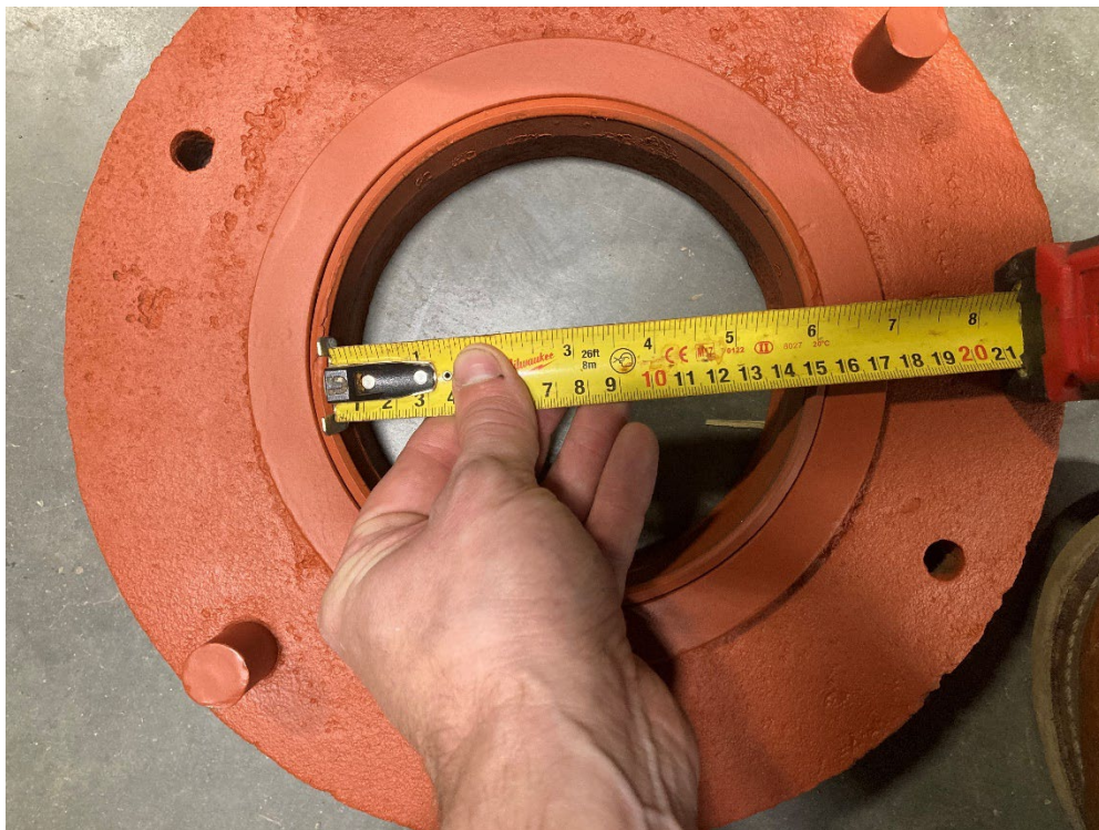
Photo 2: Slide Plate Adaptor Dimensions
