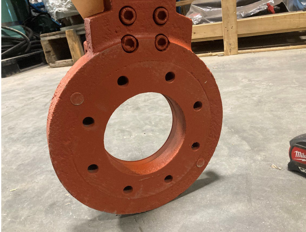
Photo 1: Existing Slide Plate Adaptor
