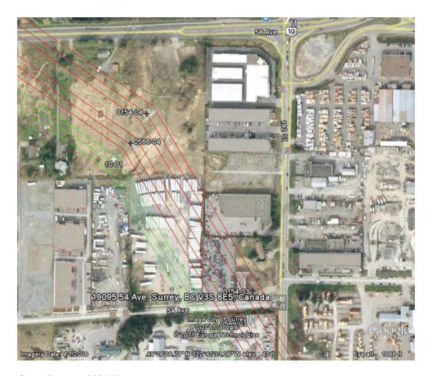
Green lines are 230 kV Red lines are 500 kV
