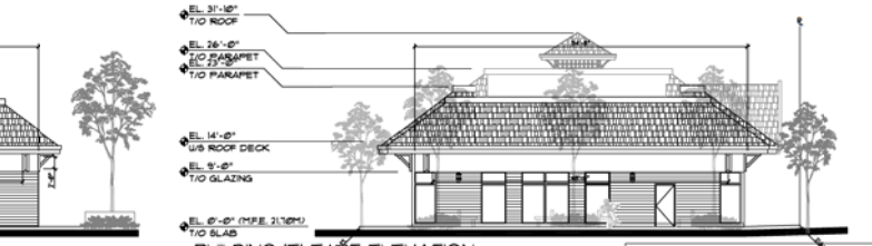
8 BUILDING 'F' EAST ELEVATION SCALE: 1/8" = 1'-0"
