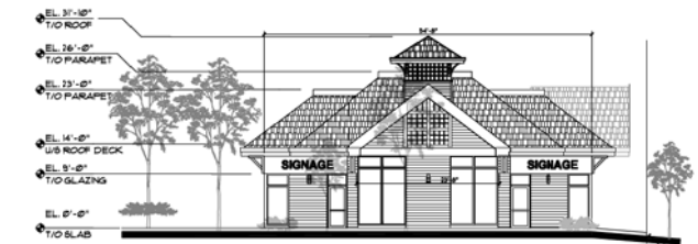
4 BUILDING 'E' EAST ELEVATION (168TH ST.) SCALE: 1/8" = 1'-0"
