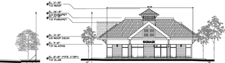
6 BUILDING 'F' WEST ELEVATION SCALE: 1/8" = 1'-0"
