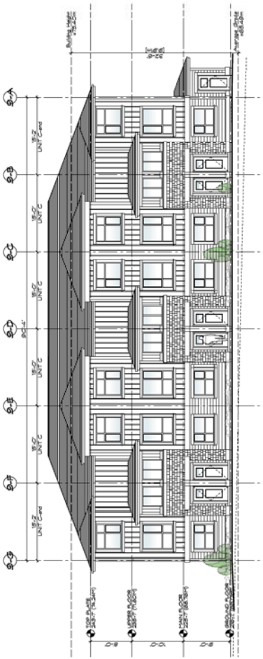
1 BUILDING 9 - EAST (FRONT) ELEVATION SCALE 1/8" = 1'-0"
