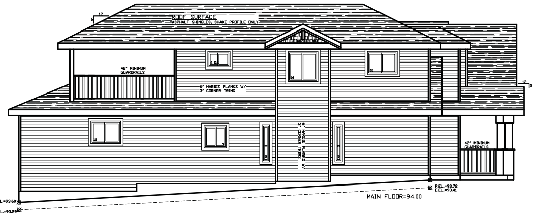
LEFT ELEVATION WALL FACE AREA=983 sq.ft ALLOWABLE AREA @8%=78.64 sq.ft ACTUAL AREA=75 sq.ft
