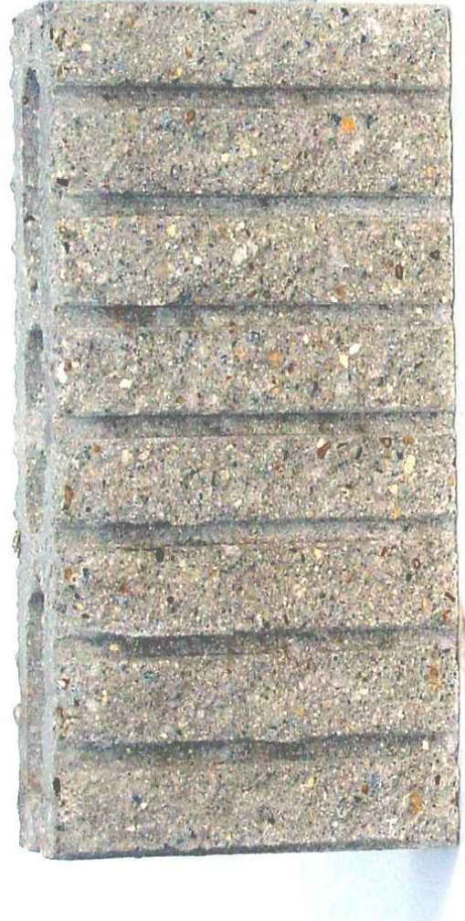
EXISTING RIBBED CONCRETE BLOCK
