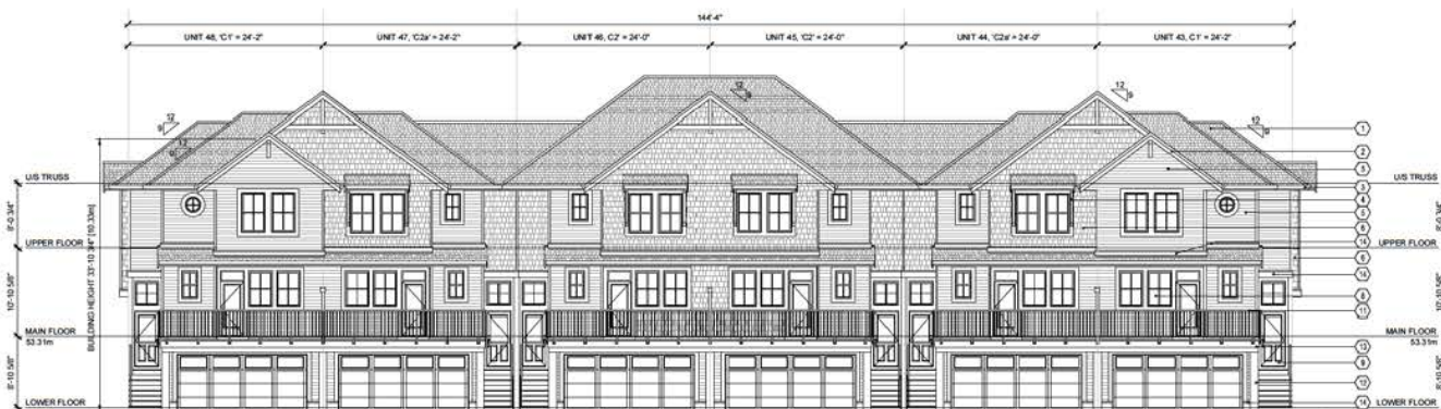
BUILDING 13 - SOUTH ELEVATION SCALE: 1/8"=1'-0"
