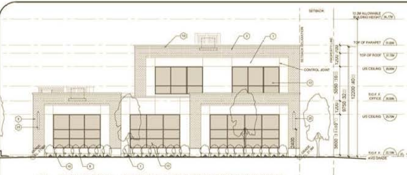
1 BUILDING A - NORTH ELEVATION (64TH AVENUE) SCALE: 1:100
