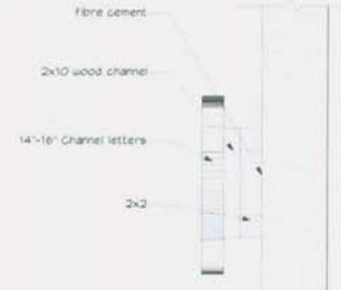
FASCIA SIGN SECTION DETAIL
