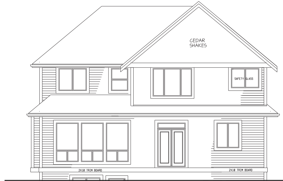
REAR FACADE WITH OFFSET AND ROOF SKIRT
