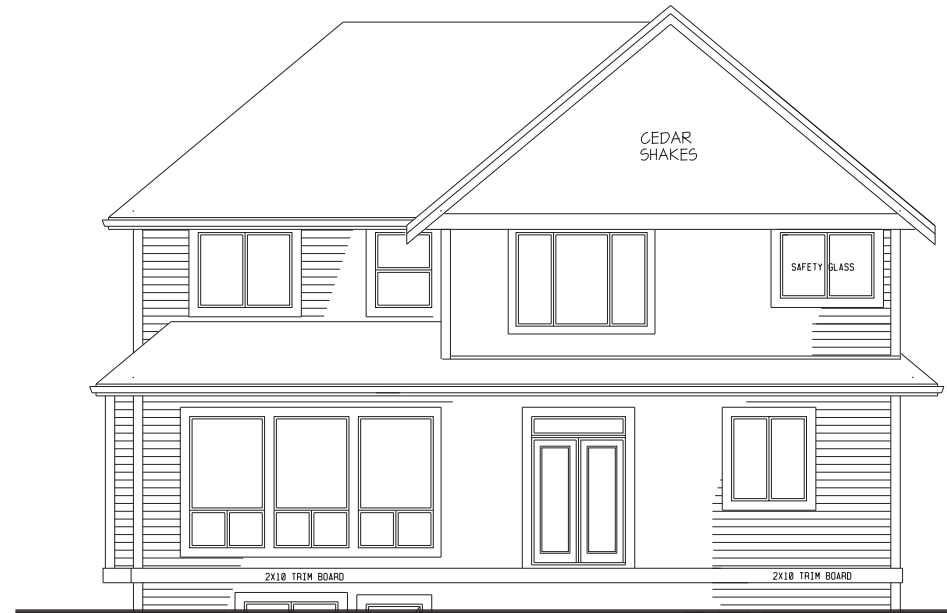
REAR FACADE WITH OFFSET AND ROOF SKIRT
