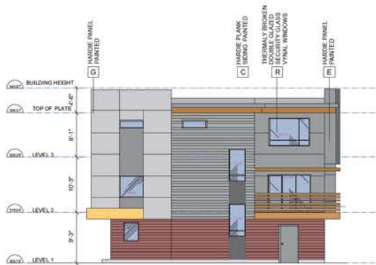
NORTH ELEVATION BUILDING B
