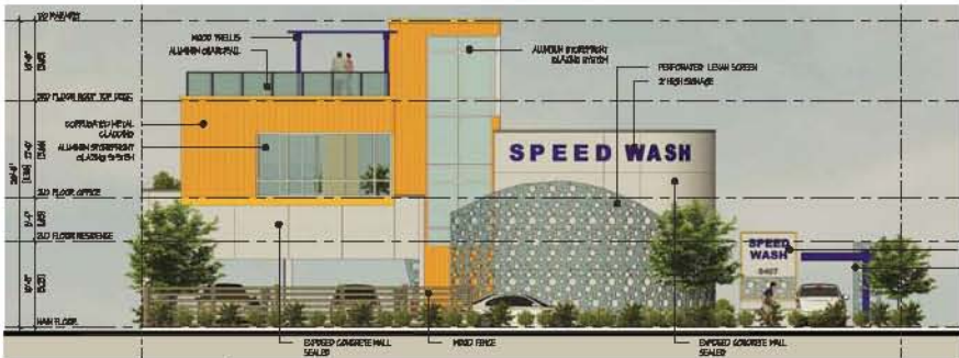
SOUTH ELEVATION (84TH AVENUE) SCALE 3/8" = 1'-0"
