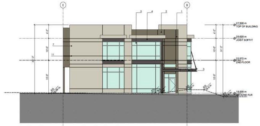
EAST ELEVATION - BLDG 100 1/8"=1'0"
