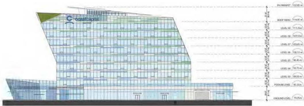
1 BUILDING A - SOUTH ELEVATION SCALE 1:300
