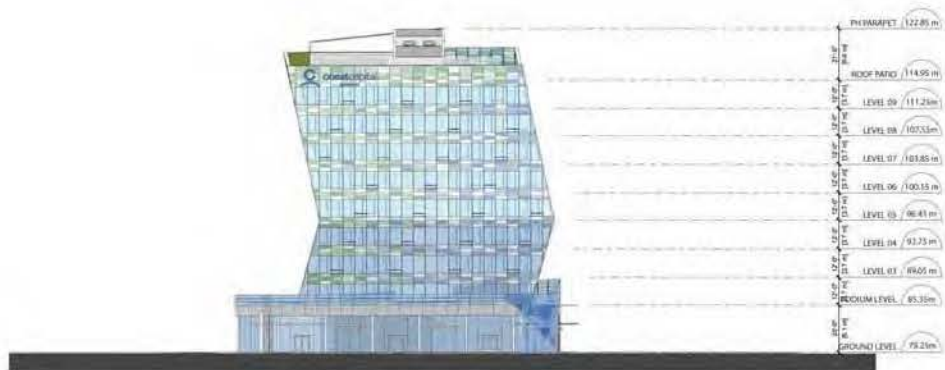
2 BUILDING A - EAST ELEVATION SCALE 1:300
