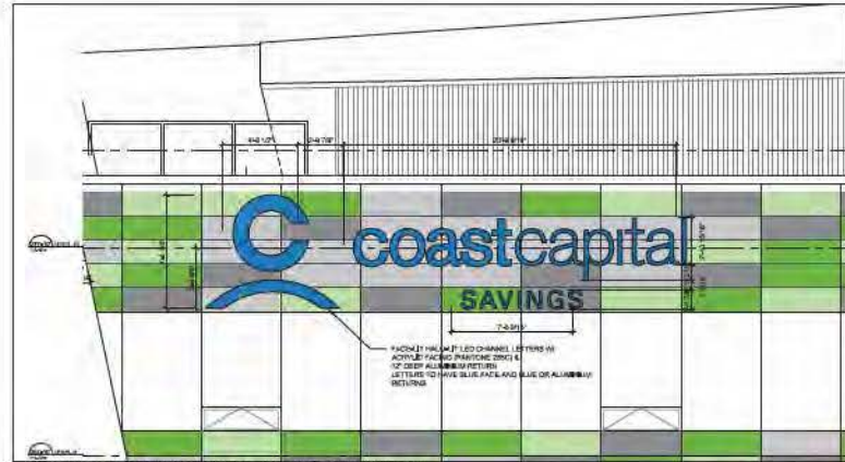
2 FASCIA SIGNAGE (TYPE 1) EAST ELEVATION SCALE: 1/4" = 1'-0"
