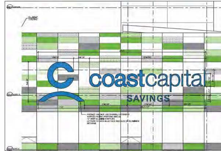
4 FASCIA SIGNAGE (TYPE 2) WEST ELEVATION SCALE: 1/4" = 1'-0"
