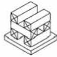
CRIB BLOCKING A 6x6x18 LONG LUMBERS ON 24x24x3 PRESSURE TREATED WOOD PADS OR CONCRETE BLOCK
