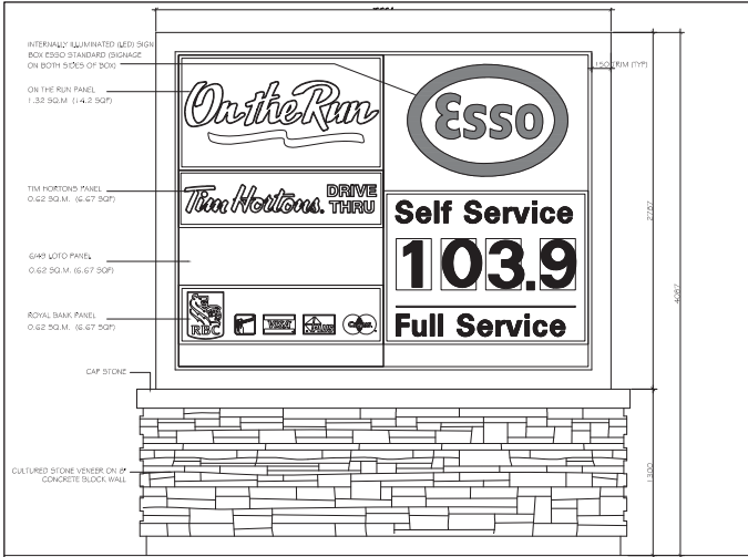
1 FREE STANDING SIGN ELEVATION DET 3 SCALE: 1:20
