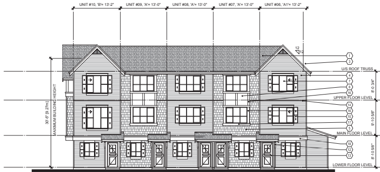
BUILDING 2 - EAST ELEVATION SCALE: 1/8" = 1'-0"
