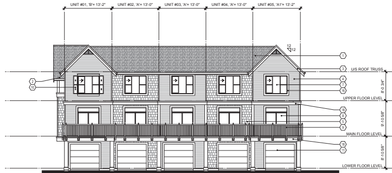
BUILDING 1 - WEST ELEVATION SCALE: 1/8" = 1'-0"
