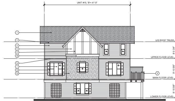
BUILDING 4 - SOUTH ELEVATION SCALE: 1/8" = 1'-0"
