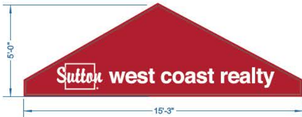
5'-0" x 15'-3" S/F ILLUMINATED FASCIA SIGN BACKGROUND, CABINET & RETAINER TO MATCH PANTONE #187C RED, WHITE GRAPHICS
