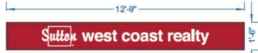
1'-6" x 12'-9" S/F ILLUMINATED FASCIA SIGN BACKGROUND, CABINET & RETAINER TO MATCH PANTONE #187C RED, WHITE GRAPHICS
